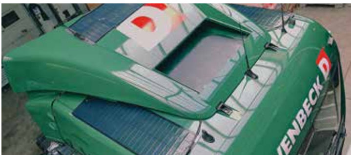
EUROPART supplies the Duvenbeck Group with the solar cells in pre-configured MIPV sets (165 Wp Mobile Integrated Photovoltaic) as well as inverters and accessories.
